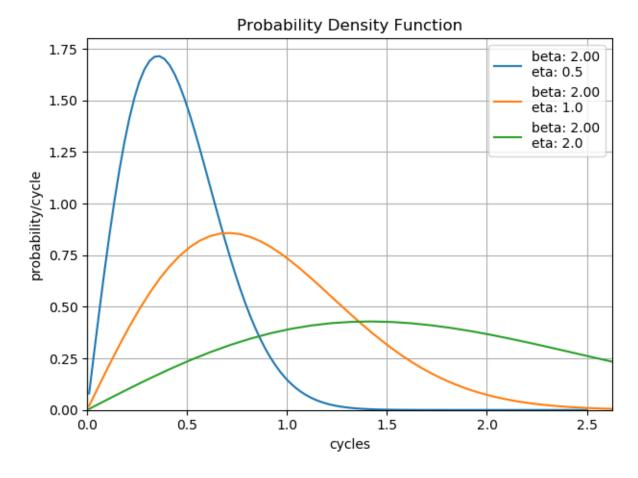
Note that changes in the scale factor keep the shape, but effectively change the length over which the distribution is 'stretched'. The hange in height is due to the property that the area under the curve must always be equal to 1.0.
