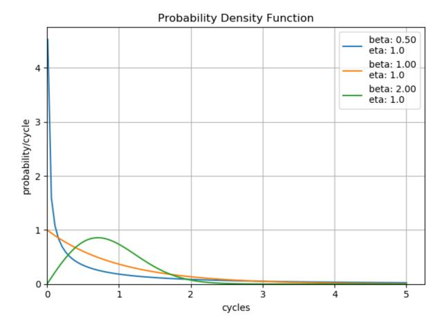
It is possible for a product to exhibit all three of these characteristics on different components. Imagine a car which has adhesives, electronics, and bearings, each of which have their own failure distributions. With careful analysis of the failure modes, it is possible to determine the individual component failure distributions, which allows the designer to potentially identify and resolve the most problematic elements of the design first.
