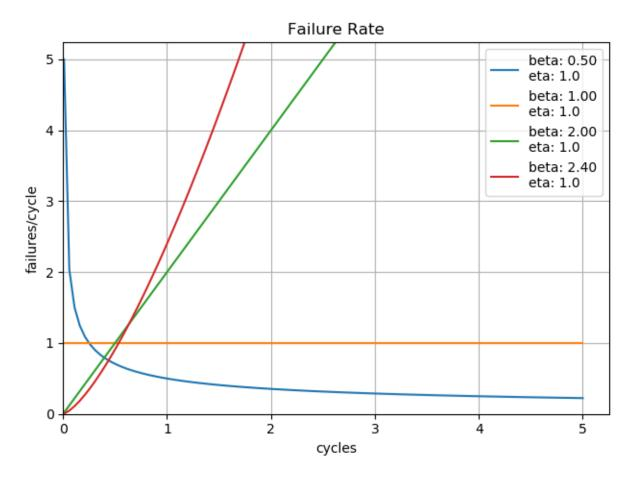
It is the combination of these three potentially different  $\beta$  characteristics that gives rise to the traditional bathtub curve commonly observed in reliability analysis. Looking closely at the plot of failure rates, one can see that a product composed of three different  $\beta$  characteristic components could begin to form an overall bathtub curve of the composite failure rates.
